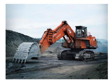
A current DYNAVIS<sup>®</sup> test project: HITACHI EX1200 crawler excavator in the Kuznetsk Basin, Russia. A hydraulic fluid formulated using DYNAVIS<sup>®</sup> technology yielded productivity growth (cbm<sup>3</sup>/h) in coal extraction measured at 7.9%.
