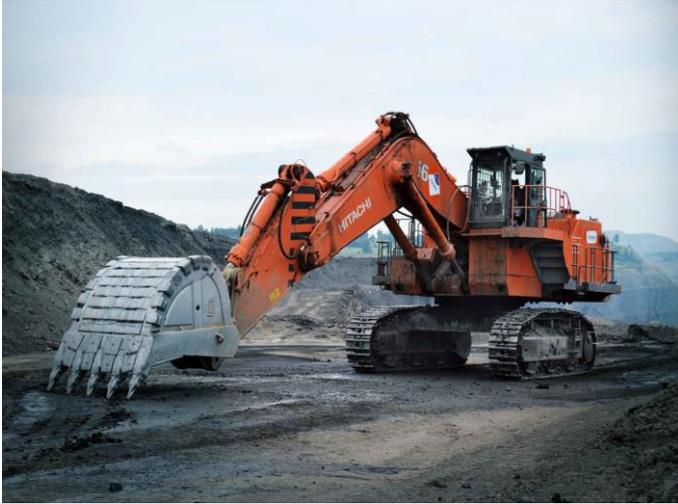
*A current DYNAVIS® test project: HITACHI EX1200 crawler excavator in the Kuznetsk Basin, Russia. A hydraulic fluid formulated using DYNAVIS® technology yielded productivity growth (cbm<sup>3</sup>/h) in coal extraction measured at 7.9%.*
